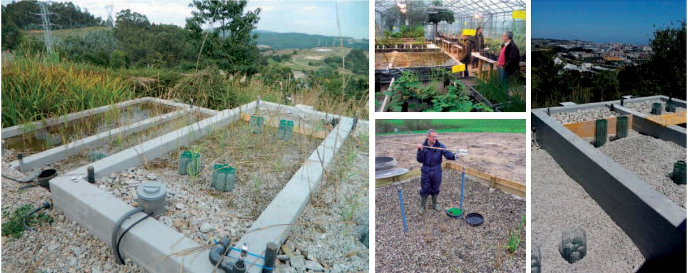
The goal of HIGHWET is to develop holistic configurations combining hydrolytic anaerobic digester (HUSB) and vertical and horizontal CWs capable of operating at high loading rate of about 20-50 g BOD/m<sup>2</sup>d (for the overall system and according the configuration), thus reducing the land requirements by a factor of 2 to 4 regarding conventional CWs.
